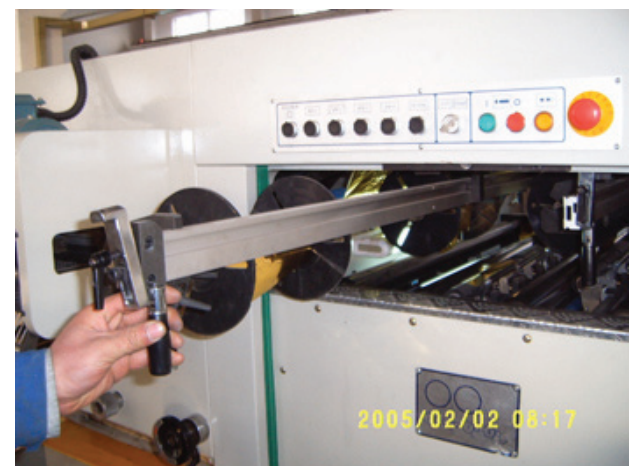
Free standing rewriter with 6 tension axles
